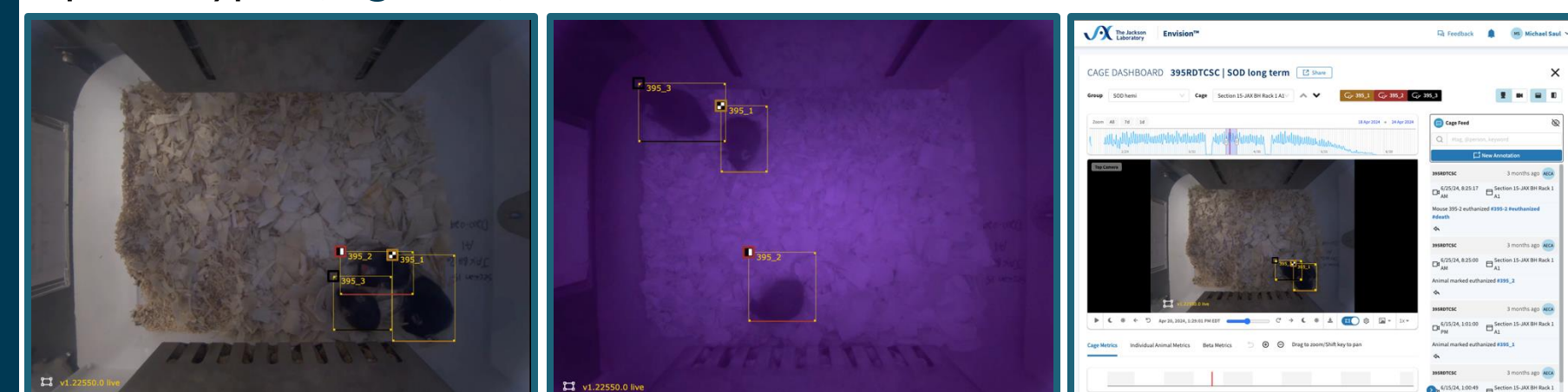
Figure 1. JAX Envision™ collects video in the light (left) and dark (center) cycles and sends the results through a set of machine learning algorithms that are reported through a cloud-based user interface.
